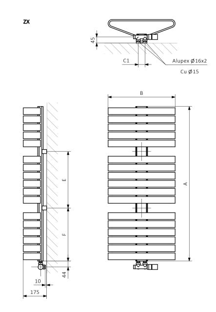
$\begin{array}{lll} A-{\sf Height} & B-{\sf Width} & {\sf C1-C5-Distance\ between\ pipe\ centres} & D-{\sf Horizontal\ distance\ between\ mounting\ bracket\ centres} \\ E-{\sf Vertical\ distance\ between\ mounting\ brackets} & F-{\sf Distance\ between\ a\ mounting\ bracket\ and\ the\ bottom\ of\ the\ radiator} \end{array}$
