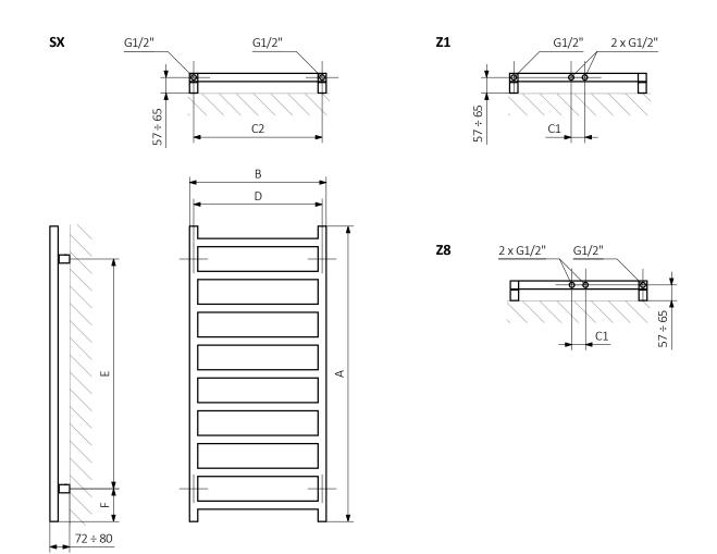
$\begin{array}{lll} A-{\sf Height} & B-{\sf Width} & {\sf C1-C5-Distance\ between\ pipe\ centres} & D-{\sf Horizontal\ distance\ between\ mounting\ bracket\ centres} \\ E-{\sf Vertical\ distance\ between\ mounting\ brackets} & F-{\sf Distance\ between\ a\ mounting\ bracket\ and\ the\ bottom\ of\ the\ radiator} \end{array}$
