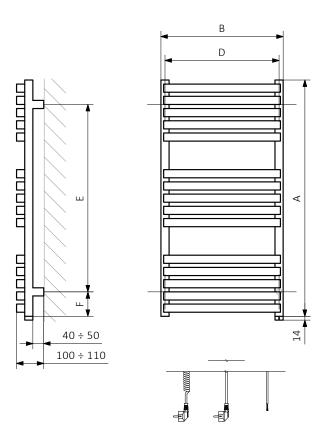
A — Height B — Width C1-C5 — Distance between pipe centres D — Horizontal distance between mounting bracket centres E — Vertical distance between mounting brackets F — Distance between a mounting bracket and the bottom of the radiator
