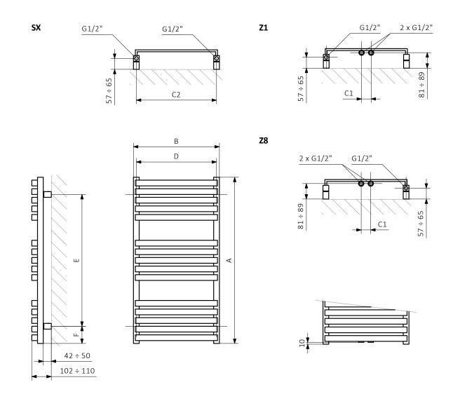
$\begin{array}{lll} A - \mbox{Height} & B - \mbox{Width} & \mbox{C1-C5} - \mbox{Distance between pipe centres} & \mbox{D} - \mbox{Horizontal distance between mounting bracket centres} \\ E - \mbox{Vertical distance between mounting brackets} & \mbox{F} - \mbox{Distance between a mounting bracket and the bottom of the radiator} \\ \end{array}$
