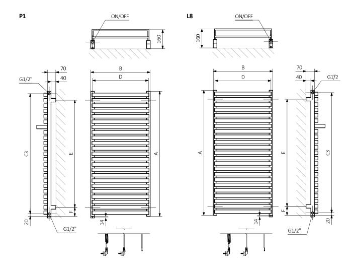
$A- Height \quad B- Width \quad C1-C5- Distance \ between \ pipe \ centres \quad D- Horizontal \ distance \ between \ mounting \ bracket \ centres \\ E- Vertical \ distance \ between \ mounting \ brackets \quad F- Distance \ between \ a \ mounting \ bracket \ and \ the \ bottom \ of \ the \ radiator$
