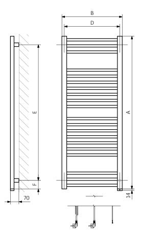
${\rm A-Height}\quad {\rm B-Width}\quad {\rm C1-C5-Distance~between~pipe~centres}\quad {\rm D-Horizontal~distance~between~mounting~bracket~centres}$ E — Vertical distance between mounting brackets F — Distance between a mounting bracket and the bottom of the radiator
