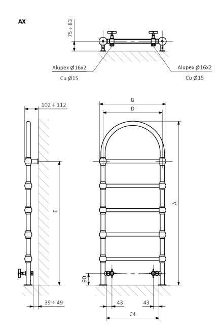
$\begin{array}{lll} A-{\sf Height} & B-{\sf Width} & {\sf C1-C5-Distance\ between\ pipe\ centres} & D-{\sf Horizontal\ distance\ between\ mounting\ bracket\ centres} \\ E-{\sf Vertical\ distance\ between\ mounting\ brackets} & F-{\sf Distance\ between\ a\ mounting\ bracket\ and\ the\ bottom\ of\ the\ radiator} \end{array}$
