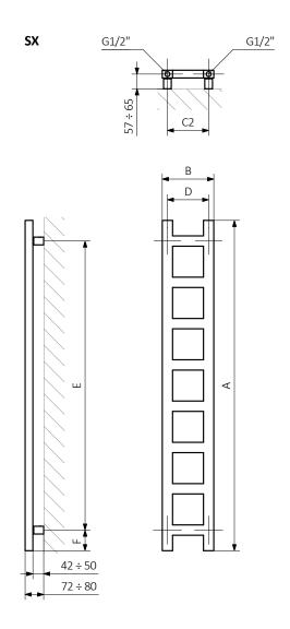
$A-Height \quad B-Width \quad C1-C5-Distance \ between \ pipe \ centres \quad D-Horizontal \ distance \ between \ mounting \ bracket \ centres \\ E-Vertical \ distance \ between \ mounting \ brackets \quad F-Distance \ between \ a \ mounting \ bracket \ and \ the \ bottom \ of \ the \ radiator$
