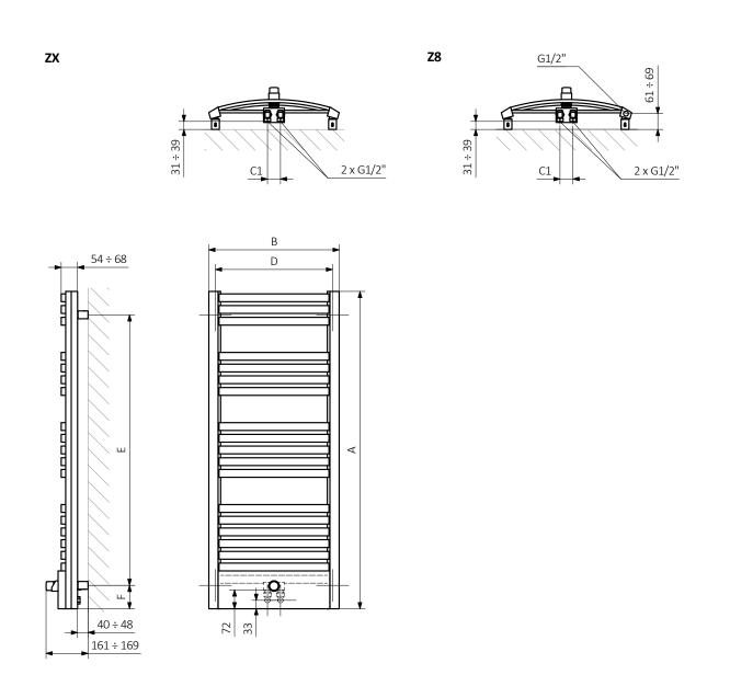
$\begin{array}{lll} A-Height & B-Width & C1-C5-Distance between pipe centres & D-Horizontal distance between mounting bracket centres \\ E-Vertical distance between mounting brackets & F-Distance between a mounting bracket and the bottom of the radiator \\ \end{array}$
