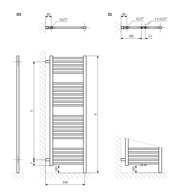
$\begin{array}{lll} A-{\sf Height} & B-{\sf Width} & {\sf C1-C5-Distance\ between\ pipe\ centres} & D-{\sf Horizontal\ distance\ between\ mounting\ bracket\ centres} \\ E-{\sf Vertical\ distance\ between\ mounting\ brackets} & F-{\sf Distance\ between\ a\ mounting\ bracket\ and\ the\ bottom\ of\ the\ radiator} \end{array}$
