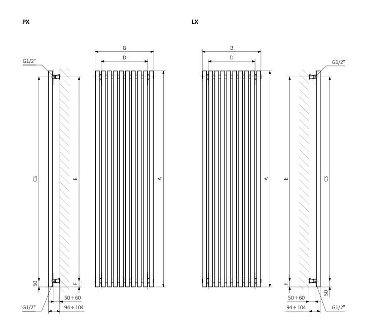
$\begin{array}{lll} A-{\sf Height} & B-{\sf Width} & {\sf C1-C5-Distance\ between\ pipe\ centres} & D-{\sf Horizontal\ distance\ between\ mounting\ bracket\ centres} \\ E-{\sf Vertical\ distance\ between\ mounting\ brackets} & F-{\sf Distance\ between\ a\ mounting\ bracket\ and\ the\ bottom\ of\ the\ radiator} \end{array}$
