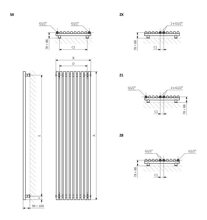
$\begin{array}{lll} A-{\sf Height} & B-{\sf Width} & {\sf C1-C5-Distance\ between\ pipe\ centres} & D-{\sf Horizontal\ distance\ between\ mounting\ bracket\ centres} \\ E-{\sf Vertical\ distance\ between\ mounting\ brackets} & F-{\sf Distance\ between\ a\ mounting\ bracket\ and\ the\ bottom\ of\ the\ radiator} \end{array}$
