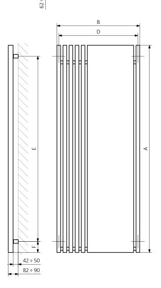
$A- Height \quad B- Width \quad C1- C5- Distance \ between \ pipe \ centres \quad D- Horizontal \ distance \ between \ mounting \ bracket \ centres \\ E- Vertical \ distance \ between \ mounting \ brackets \quad F- Distance \ between \ a \ mounting \ bracket \ and \ the \ bottom \ of \ the \ radiator$
