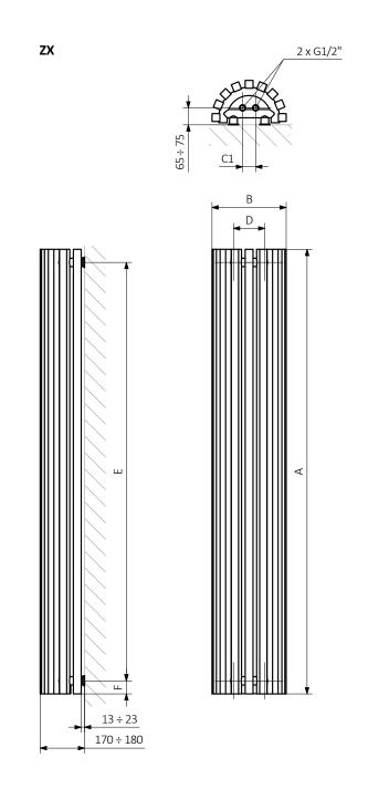
$\begin{array}{lll} A-Height & B-Width & C1-C5-Distance \ between \ pipe \ centres & D-Horizontal \ distance \ between \ mounting \ bracket \ centres \\ E-Vertical \ distance \ between \ mounting \ brackets & F-Distance \ between \ a \ mounting \ bracket \ and \ the \ bottom \ of \ the \ radiator \\ \end{array}$
