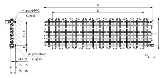
$A-Height \quad B-Width \quad C1-C5-Distance \ between \ pipe \ centres \quad D-Horizontal \ distance \ between \ mounting \ bracket \ centres \\ E-Vertical \ distance \ between \ mounting \ brackets \quad F-Distance \ between \ a \ mounting \ bracket \ and \ the \ bottom \ of \ the \ radiator$
