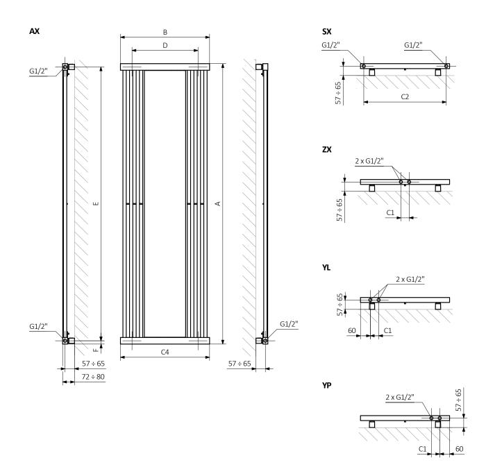
$\begin{array}{lll} A-{\sf Height} & B-{\sf Width} & {\sf C1-C5-Distance\ between\ pipe\ centres} & D-{\sf Horizontal\ distance\ between\ mounting\ bracket\ centres} \\ E-{\sf Vertical\ distance\ between\ mounting\ brackets} & F-{\sf Distance\ between\ a\ mounting\ bracket\ and\ the\ bottom\ of\ the\ radiator} \end{array}$
