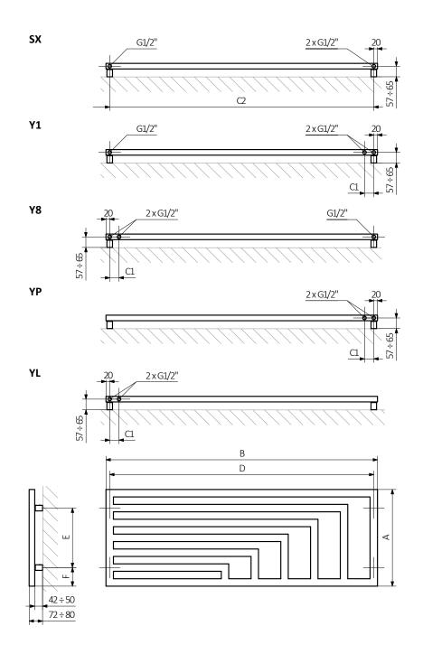
$A-Height \quad B-Width \quad C1-C5-Distance \ between \ pipe \ centres \quad D-Horizontal \ distance \ between \ mounting \ bracket \ centres \\ E-Vertical \ distance \ between \ mounting \ brackets \quad F-Distance \ between \ a \ mounting \ bracket \ and \ the \ bottom \ of \ the \ radiator$
