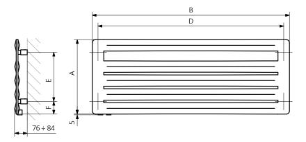
$\begin{array}{lll} A-{\sf Height} & B-{\sf Width} & {\sf C1-C5-Distance\ between\ pipe\ centres} & D-{\sf Horizontal\ distance\ between\ mounting\ bracket\ centres} \\ E-{\sf Vertical\ distance\ between\ mounting\ brackets} & F-{\sf Distance\ between\ a\ mounting\ bracket\ and\ the\ bottom\ of\ the\ radiator} \end{array}$
